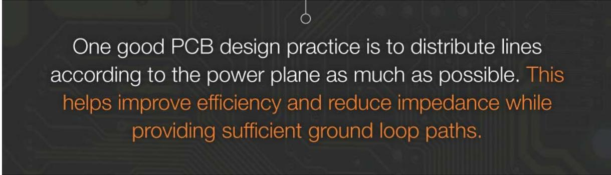
One good PCB design practice is to distribute lines according to the power plane as much as possible. This helps improve efficiency and reduce impedance while providing sufficient ground loop paths.
